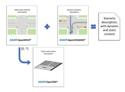
Combined all three standards provide a scenariodriven description of traffic simulation that contains static and dynamic content.
