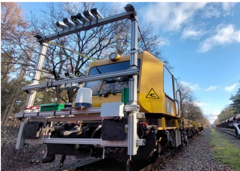
Sensor configuration on the data collection vehicle (Source: DB Netz AG)
