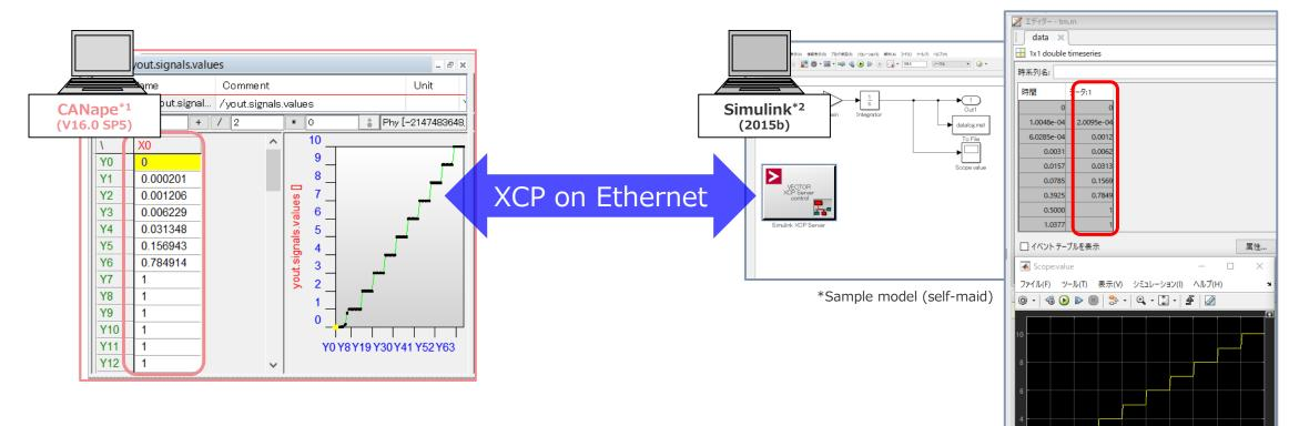
Model is executed in the simulation time (ex. executed 100 seconds in a moment). Same as the behavior of model, the result of behavior in 100 sec. is displayed on MC tool in a moment. In future we will study use cases and expand the scope using different models, for example, a vehicle model published by METI (Ministry of Economy, Trade and Industry)
