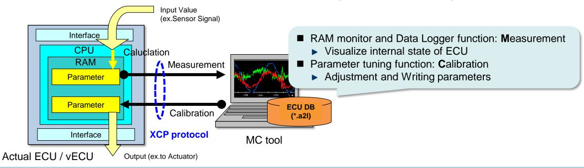
Actual ECU / vECU and MC(Measurement/Calibration) tool
