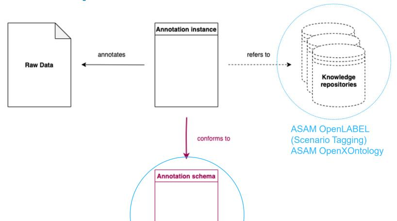
Data annotation is the process of enriching raw data, for example, data streams from multiple sensors, such as cameras, LiDAR, radar, or test scenario artifacts with additional metadata. These metadata are related to the content of the raw data, for example, static or dynamic objects populating a video, actions they are performing, or environmental conditions Additional information regarding the data may also be included.
