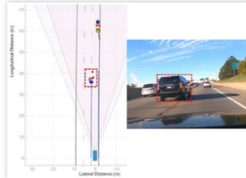
FIGURE 14 Driving case (c): cut-in vehicle with too close distance
