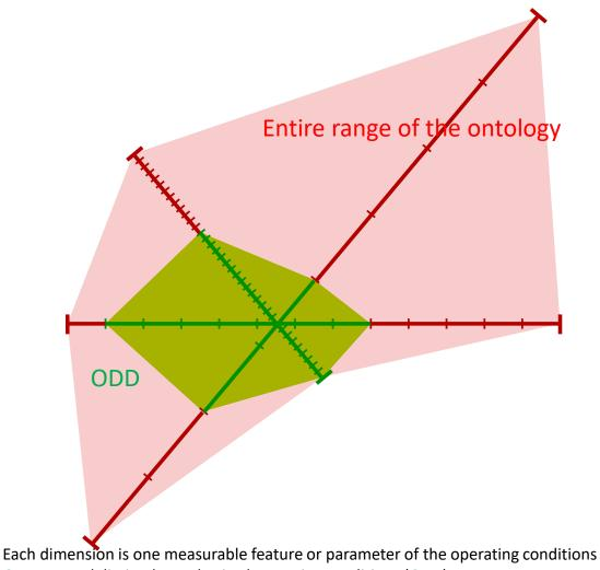
Each dimension is one measurable feature or parameter of the operating conditions Green area delimits the authorized operating conditions (ODD) Red parts are operating conditions not intended for AD operation (i.e. outside ODD)
