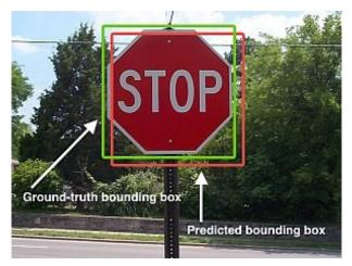
How well does the predicted bounding box match the real bounding box?
