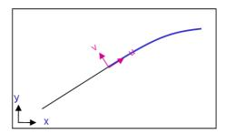
NOTE: In order to stick to the start point and orientation according to the <geometry> node, the parameters a and b will have to be zero. Providing non-zero values for these parameters will lead to a shift and rotation of the s/t co-ordinates according to the following figure:
