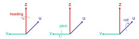
The local system can only be positioned in track space by providing the full track co-ordinates and orientation of its origin.
