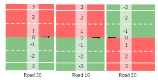
Road 10 is directly linked to road 20 and road 30. The cross sections of all roads are identical, however the directions do not match between road 10 and 20.
