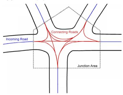
Connecting Roads are also modeled as roads according to the rules laid out here for all other roads. They consist of reference lines with lane sections etc. Usually, in-coming roads also serve as outgoing roads, with the actual usage of a road being determined by its lanes.
