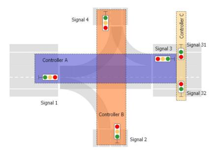
In this example, the signals 31 and 32 are controlled by an additional controller "Controller C". If corresponding pedestrian signals existed at the location of "Signal 1", they could also be controlled by "Controller C".
