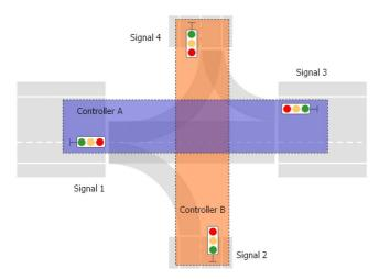
It is recommended to assign synchronous signals of same type to identical controllers instead of having one controller for each signal. So, in the example above, both through-directions will be controlled by individual controllers.
