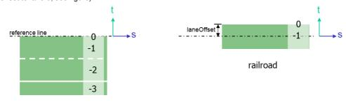
**NOTE:** For railroad lines with multiple parallel tracks (typically dual-track layout), it is mandatory to use one discrete track per direction instead of adding railroad lanes to an existing track. It is also recommended to provide individual reference lines (each bearing exactly one lane) for rail-based vehicles even in areas of shared use with road vehicles.
