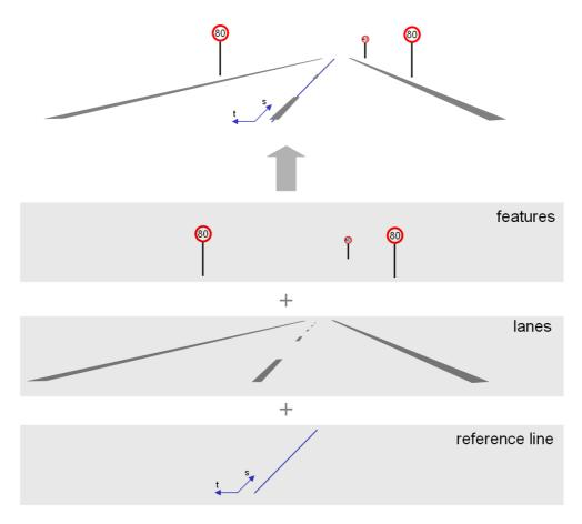
All roads consist of a reference line which defines the basic geometry (arcs, straight lines etc.). Along the reference line, various properties of the road can be defined. These are, e.g. elevation profile, lanes, traffic signs etc. Roads can be linked to each other either directly (when there is only one connection possible between two given roads) or via junctions (when more than one connection is possible from a given road to other roads).
