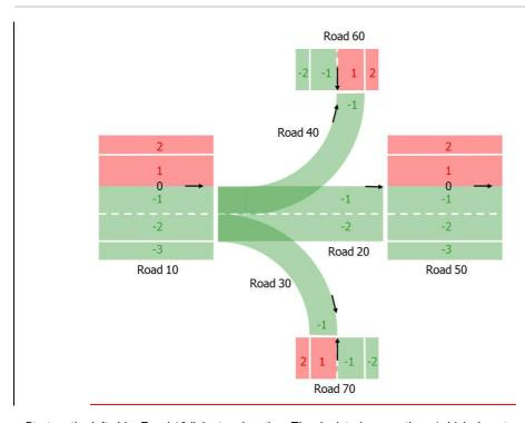
Start on the left side: Road 10 links to a junction. The depicted connections (which do not represent the entire connection matrix) allow for the following ways to navigate the junction:
