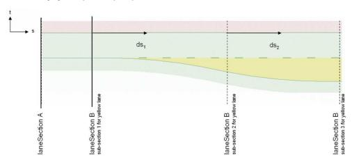
Per lane section, the number of lanes is constant. However, the properties of each lane (e.g. width, road marks, friction etc.) may change.
