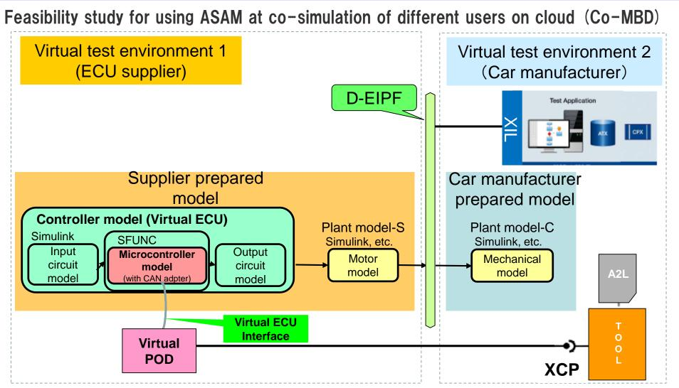
ASAM XIL : an API standard for the communication between test automation tools and test benches ASAM MCD-1 XCP : a bus-independent, master-slave communication protocol to connect ECUs with calibration systems
