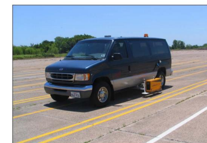
Figure 5. Typical Mobile Pavement Marking Retroreflectivity Measurement Device
