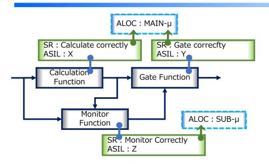
Typical expression for SC based on Function Block Diagram before SCDL
